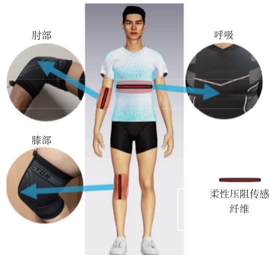
图 5 一维结构电阻应变传感器在服装上的应用 Fig. 5 One-dimensional structural resistive strain sensors for clothing applications
