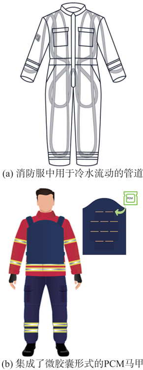
图 2 消防服中集成温度调节模块示意 Fig. 2 Schematic diagram of the integrated thermoregulation module in a firefighting clothing
