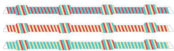
Fig.3 Thick segment colored slub yarns formed by one main roving and two auxiliary rovings and their pattern effects
