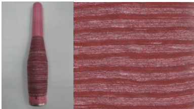
图14 段彩竹节纱粗细节段纱线及织物布面效果 Fig.14 Yarn and fabric surface effect of thick and thin colored slub yarn
