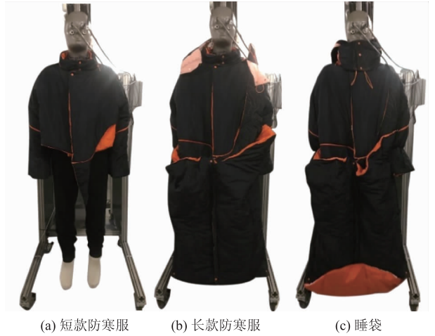
图 11 3 种着装模式暖体假人实验 Fig. 11 Experiments with three types of wearing models
