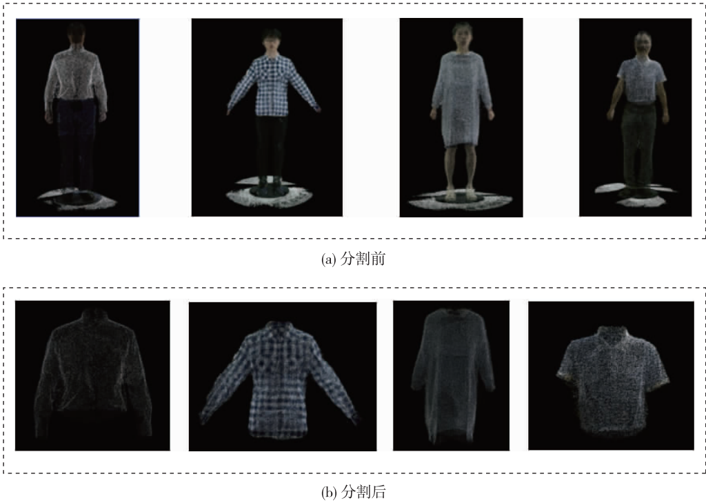
图 3 服装区域点云分割前后效果对比 Fig.3 Effect comparison before and after point cloud segmentation in clothing area
