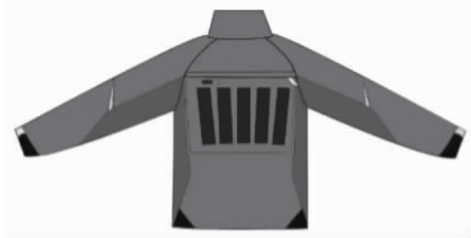
图 4 薄膜太阳能可调温发热服 Fig. 4 Thin-film solar heating suit with adjustable temperature
