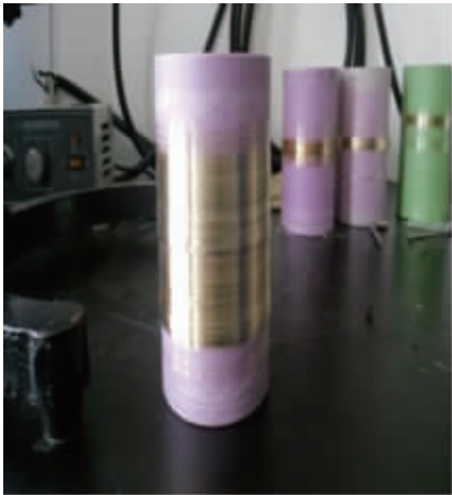
图 4 含硼量的屏蔽纤维 Fig.4 Shielding fiber containing boron
