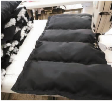
图 11 填充棉夹层绗缝 Fig. 11 Quilting technology of filled cotton interlayer
