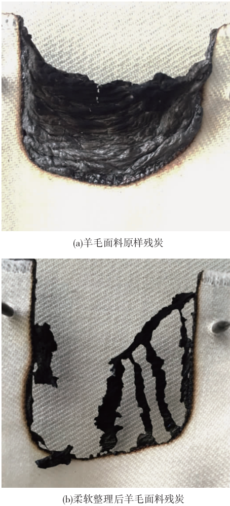
图 3 柔软整理前后羊毛面料残炭形态 Fig. 3 Morphology of carbon residue of wool fabric before and after softening finishing
